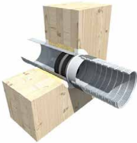
FSAeco-ST in 150 mm dwars gelamineerde houten wand
