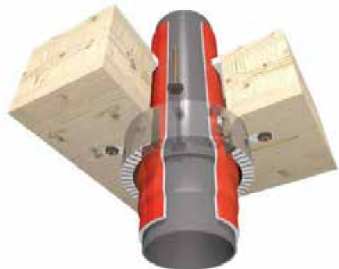
RORCOL V60 for sewage pipes with plug-in sleeve
