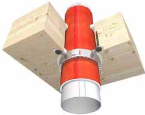
RORCOL V30 for sewage pipes with insulation
