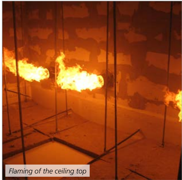
Fire load on the ceiling top
