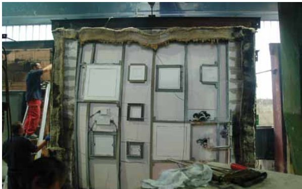
Fire load on shaft side (i→o)
