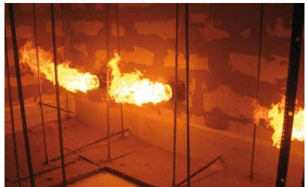
Fire load on top of ceiling (a→b)
