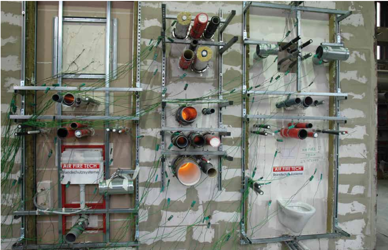
Fire resistance testing as per European standards including concealed WC cistern installed in a shaft wall
