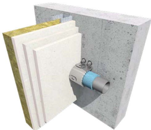
RORCOL V60 mounted as Omega-application, on the wall
