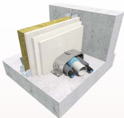
RORCOL AV60 mounted as Omega-application, on the top side of the floor
